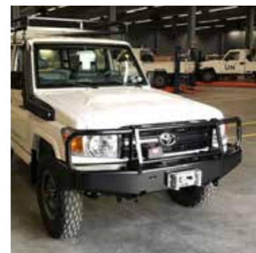
Pare-buffle renforcé, prise treuil Bullbar, Heavy Duty incl. winchbumper LC78/LC79/LC76 Ref. 20TF0030
