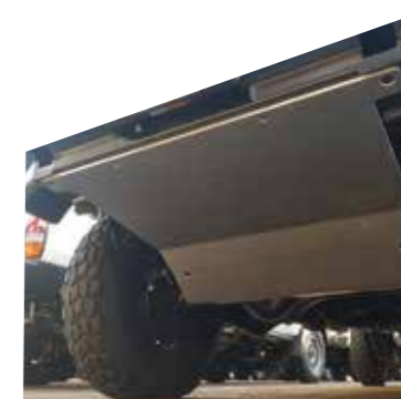
Plaque de protection avant - sans Pare-buffle complet Front skid plate without bullbar/ winchbumper LC76,LC78,LC79 Ref. 20TF0055
