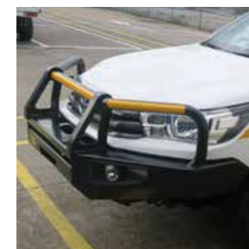
Pare-buffle renforcé, prise treuil, clignotants, feux antibrouillard Bullbar, Bullbar, Heavy Duty incl. winchbumper, turning lights, fog lights HILUX D/C, S/C Ref. 20TF0023
