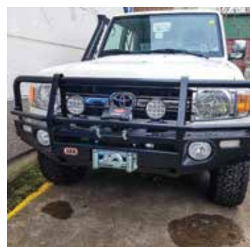
Pare-buffle renforcé, prise treuil, clignotants, feux antibrouillard Bullbar, Heavy Duty incl. winchbumper, turning lights, fog lights, wide body LC76 LX Ref. 20TF0027
