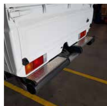
Installation du pare-choc arrière d'origine Original rear bumper mounting LC79 Ref. 20TF0084
