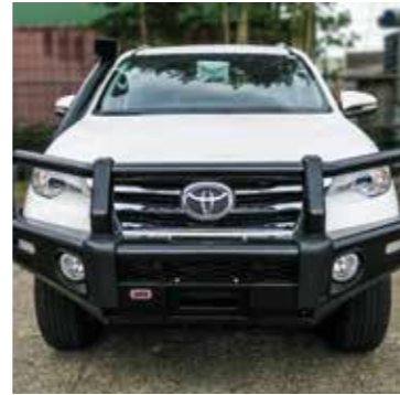
Pare-buffle renforcé, prise treuil, clignotants, feux antibrouillard Bullbar, Heavy Duty incl. winchbumper, turning lights, fog lights FORTUNER Ref. 20TF0082
